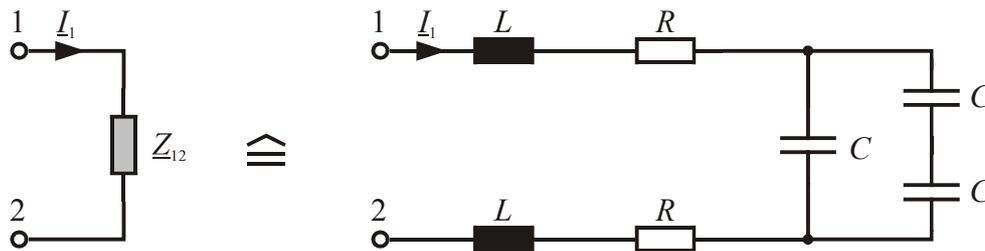
$$\underline{I}_1 = \frac{\underline{U}_{12}}{\underline{Z}_{12}} = \frac{U_0}{2R + 2(j\omega L) + \frac{1}{1,5(j\omega C)}} = \frac{230 \text{ V}}{60 \Omega + j80 \Omega - j50 \Omega} = 3,43 \text{ A} \cdot e^{-j26,6^\circ}$$
